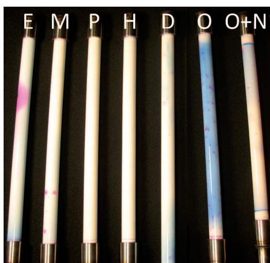
Figure 5.8. Overview of the hybrid silica membranes after the test in the dye solution
