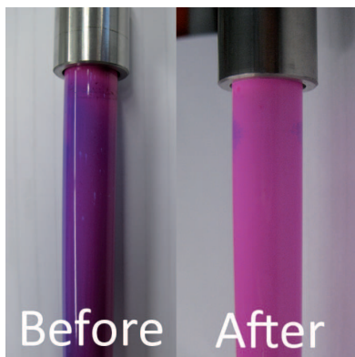
Figure 5.7. Pictures of the \gamma\text{-Al}_2\text{O}_3 support after the measurement in the acetone/dye mixture before (left) and after the cleaning with acetone (right)
